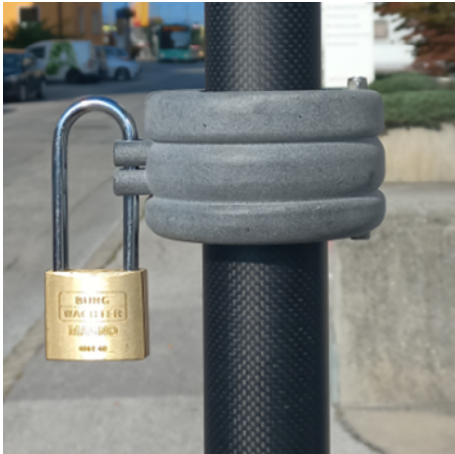
Lowest mast element secured with the mast lock.
