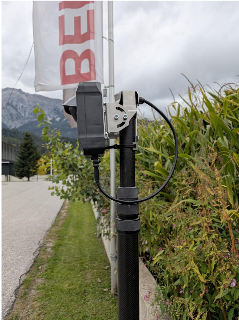
Detector mounted and secured on the telescopic mast with the power cable connected.
