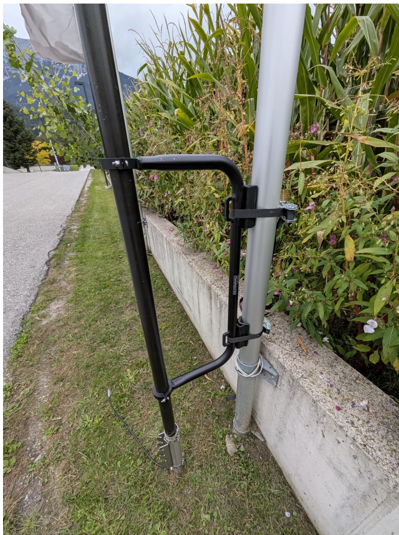
Telescopic mast secured to fixed infrastructure with tensioning straps.
